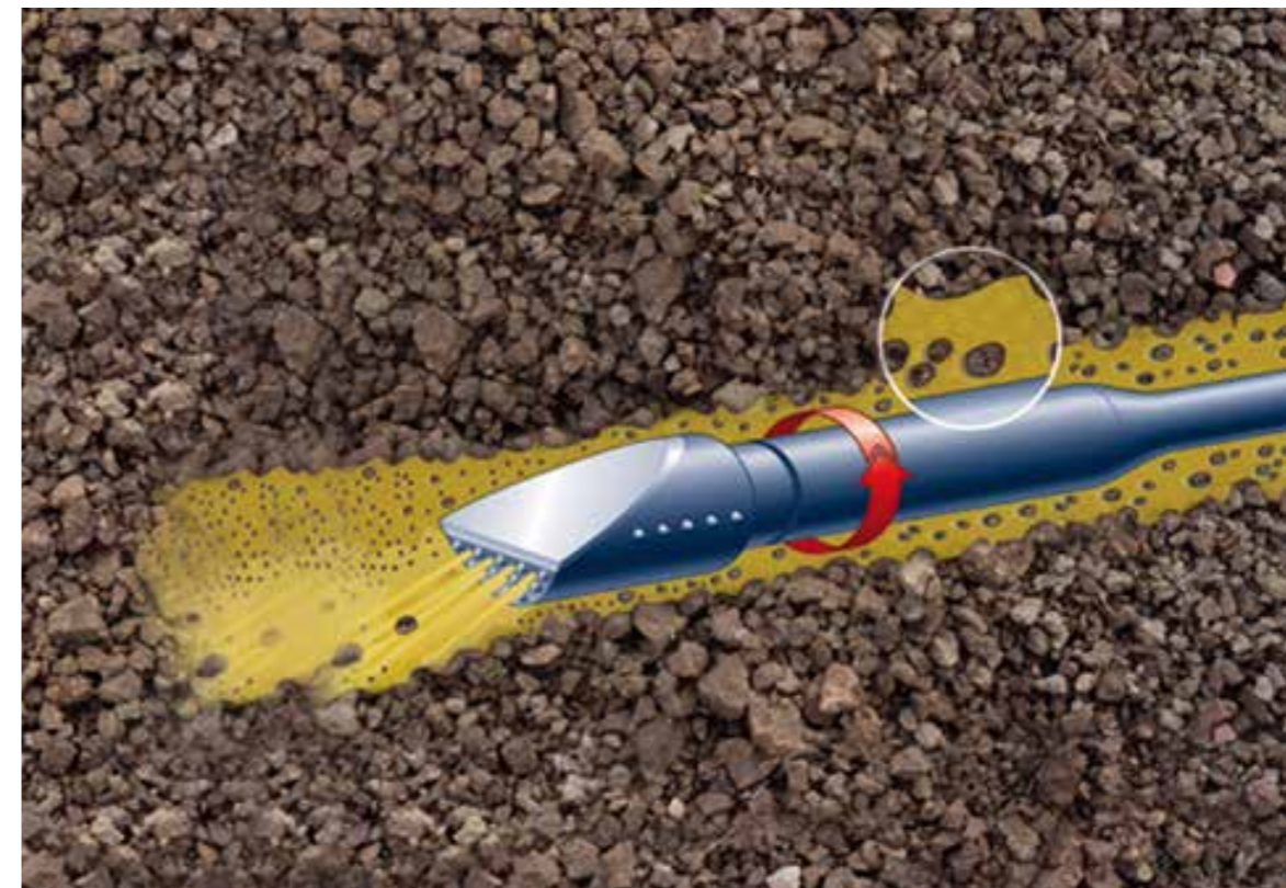
The bore hole is mainly supported by the Bentonite drilling fluid which continuously discharges the bore spoils the bore head has cut free.
