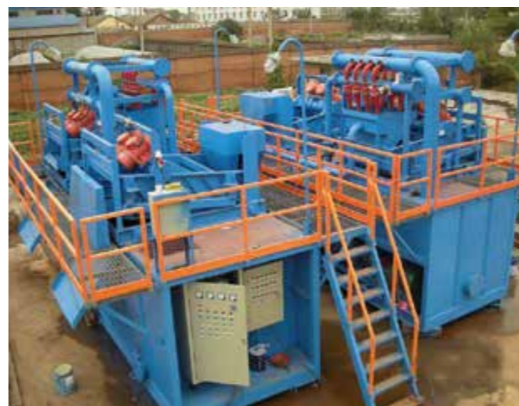
Picture left: Hydrocyclones for the separation of the sand/silt grain proportion in construction site applications.
