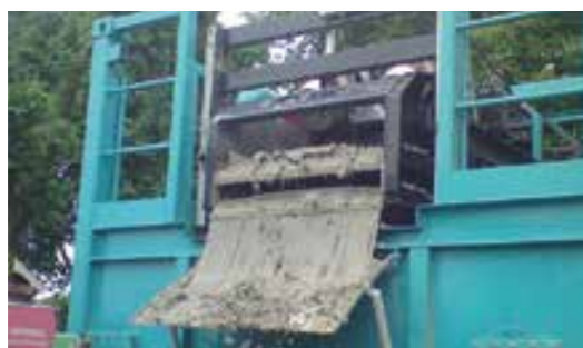
Picture above: Recycling unit with double-deck vibrating screens (shaker) for optimal separation of coarse solids from the drilling fluid.
